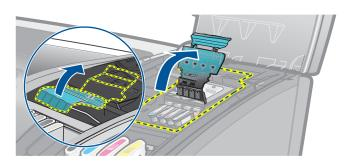
4 Lift up the handle of the printhead and use it to pull the printhead straight up and out of its slot.
